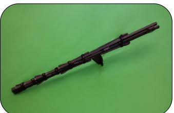
The TDLP100X5 is a broadband log periodic antenna that covers the entire band of 100-520 MHz. It is designed to achieve the maximum gain with minimum size and robust construction for harsh environments. The TDLP100X5 has folding elements for quick setup and removal.
