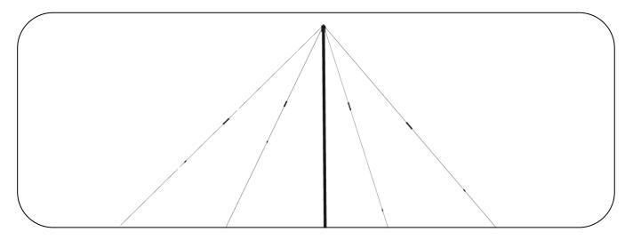
The HF Tactical Deployable Backpack "Spider Web" antenna is designed to be a light weight, single man carry, and erectable fan dipole for all radios within the 2-30 MHz band. The antenna is highly adaptable in a tactical environment and can be erected and in operation within minutes by a single operator. The center matching network can be hung from a tree, eaves of a building, fiberglass mast, or places atop large builders or mounds of earth.
