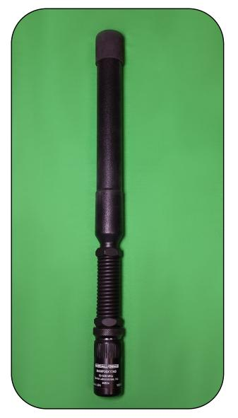
The MAMP30X17AB broadband monopole antenna is designed to be used in military or commercial, vehicular or marine applications where low profile and reliability are needed most. This antenna works with all radios within the 30-520 MHz band with a VSWR of less than 2.5:1. The base of the antenna is reinforced for rough handling
