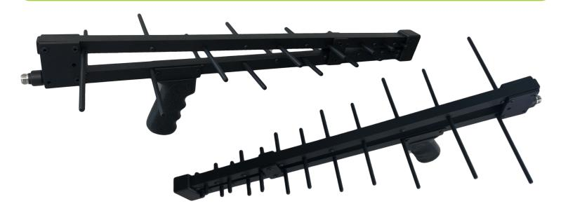
The TDLP500X5 is a broadband log periodic antenna designed to be for use as a directional handheld antenna. The robust construction of this antenna provides operational reliability in the most severe environmental conditions. The antenna has a band pass covering 500-2500 MHz with a single input.
