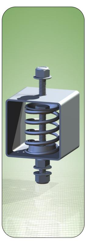
The SLH002 Spring Hanger is designed to absorb vibration to or from suspended loads. The double nut construction of the light fixture suspension bolt allows easy adjustment of up to 1/2" (12.7 mm) when installed on uneven surfaces.
