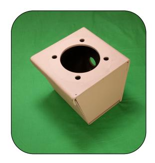
The UM012 NATO Mount allows for NATO antennas to be mounted to the top using the standard four .5" (12.7 mm) holes, equally spaced on a 4.5" (114.3 mm) dia. BHC. The lower portion also contains a hole for cable routing.
