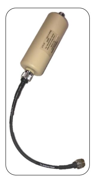
The VHF Balun is part of our Series II Communications Platform, but can be used separately to isolate a 20-88 MHz (low band) antenna from a 113-512 MHz (high band) antenna. It can also be used to feed two antenna outputs into a single radio input.
