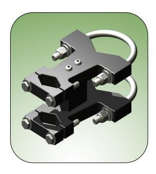
The UM008 Mast Mount is designed to mount to pole diameters up to 3" (76.2 mm) and antenna diameters from 1" (24.5 mm) to 1.5" (38.1 mm).
