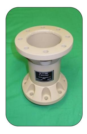
The 6" NATO Riser features the NATO Standard 8 .5" (12.77 mm) holes equally spaced on a 4.5" (114.3 mm) Dia. BHC. It is constructed of heavy duty aluminum.
