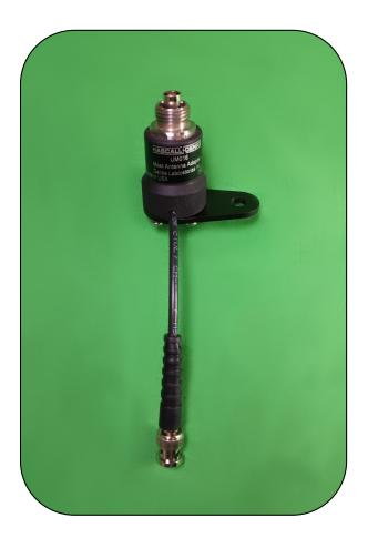
The UM016 Mast Antenna Adapter is designed to mount an antenna to the top of Denke's #1Y17100 20' Portable Mast. The UM016 can be configured for antennas with PSC-5, Type "N", TNC. BNC, and UHF connectors. See chart below for corresponding part numbers. The UM016 is mounted with standard 3/8" stainless steel hardware. The construction of the UM016 is heavy duty aluminum which is anodized and painted. A short RG-58 pigtail extends from the mount and is terminated with a BNC.
