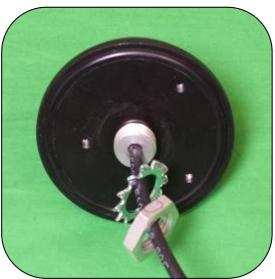
The HDM006 Roof Mount is a flush mounted base that only requires a 5/8" (16mm) drill hole for easy mounting. The mount comes with a external tooth lock washer and hex nut and 17' (5.2m) of unterminated RG-58 coax. A variety of connectors can be chosen for the antenna connection, options listed below.
