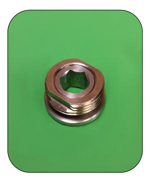
The HDM008 NMO Thru Mount is designed to be mounted on vehicle surfaces with only a single 7/8" hole and has an O-Ring for sealing against the surface. The internal hole has a hex shape to be held in place with a 1/2" Allen wrench while tightening the external part with a 15/16" wrench.
