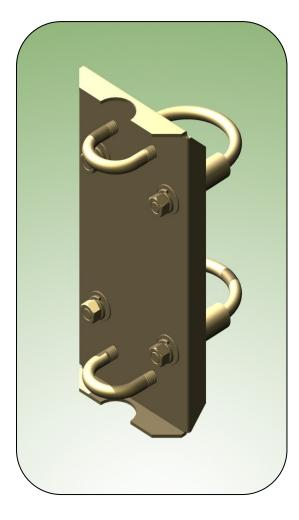
The UM003 Mounting Bracket is a pole mounted bracket commonly used for attaching our Discone or Bicone antennas. It will mount up to a 2.5" (63.5 mm) diameter mast and antennas up to 1.25" (32 mm) in diameter. It is constructed with stainless steel.
