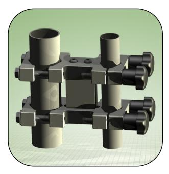
The UM007T Tactical Mount is one of our pole mounting systems that can adapt to a range of different pole diameters from 1" (24.5 mm) to 1.5" (38.1 mm). This tactical version uses quick, easy to grip knobs for fast setup and removal from the mast and permanently mounts to the antenna using bolts.
