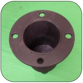
The UM011 NATO to 2" Mast Mount is an adapter that allows for NATO base antennas to be mounted on the upper ring using the standard four .5" (12.7 mm) holes, equally spaced on a 4.5" (114.3 mm) dia. BHC. The lower portion slides into the top of a mast and twist locks into position. The lower portion also contains a hole for cable routing.
