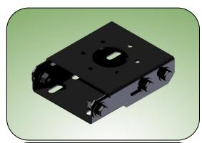
The UM002 Mounting Bracket is a versatile vehicular mount that allows tilting the antenna 90°. The bolt hole spacing pattern is 6 holes equally spaced on a 3-1/16" BHC. The mount is constructed with stainless steel for corrosion resistance.
